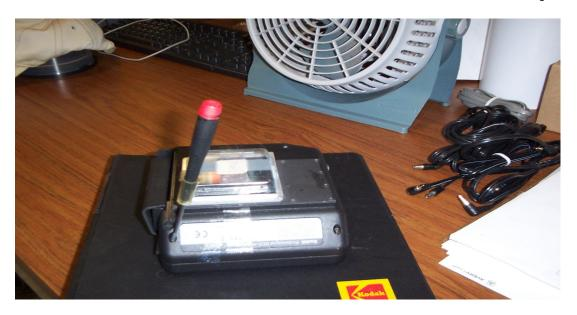
2) Flip over the Camera and remove the two SCSI silver screws and the four black screws that are located at the back side:
