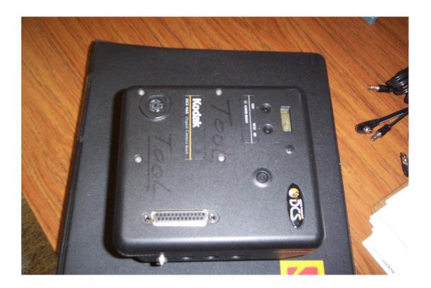
3) Holding the top cover upside DOWN so the switches will not disappear separate the top and the bottom pieces:
