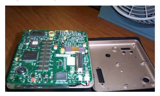
4) Remove the Battery connector from the PCB board. Back right side. And remove the two silver screws from the blades covering the Battery and slowly remove the old battery. Follow the reverse procedure to install the new one:
